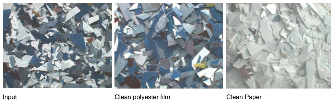
Figure 13 Separated X ray film - a suitable application for the CBS separator
