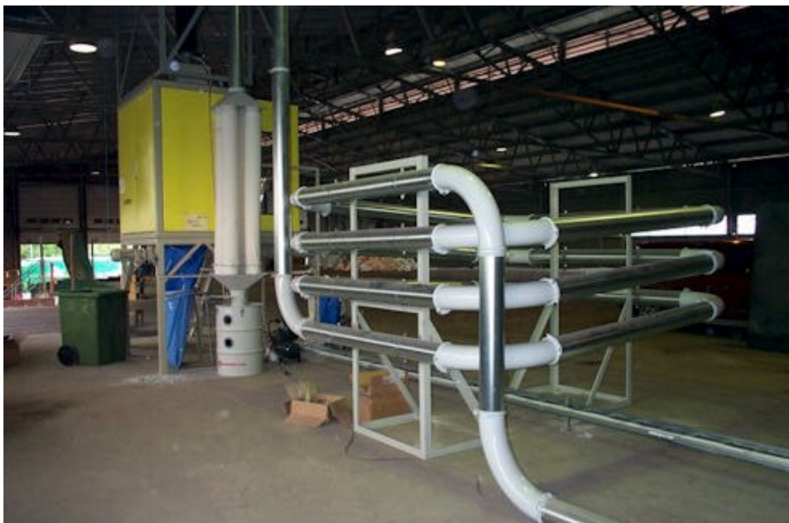
Figure 6. PE-PP separation plant built at Ragn-Sells (Sweden)
