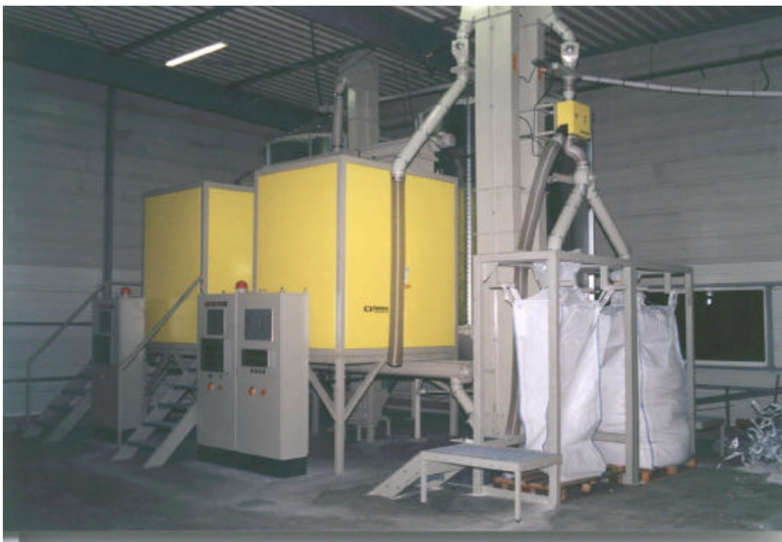
Figure 9. The Hamos EKS used for recycling of PVC windows. This unit has been supplied with complete material logistics
