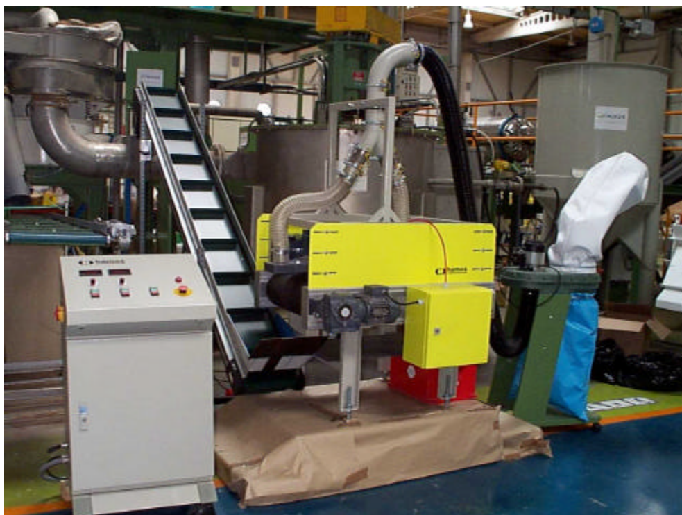
Figure 5 a) LBS separator for separating plastic from tetrabrik
